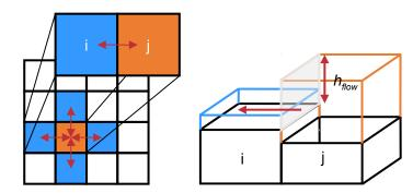
Representation of flow between cells in LISFLOOD-FP
